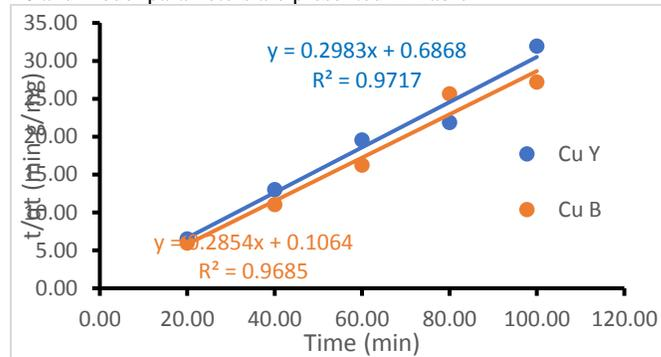
**Figure 16:** Pseudo second order Model Fit of Copper ions onto *Bacillus Circulans* and *Saccharomyces Cerevisiae*
