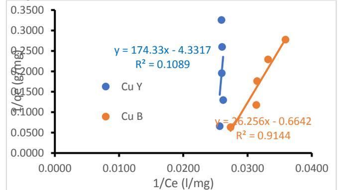
**Figure 13:** Langmuir Model Fitness for Copper ions onto *Bacillus Circulans* and *Saccharomyces Cerevisiae*
