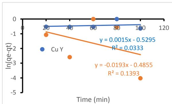
**Figure 15:** Pseudo first order Model Fit of Copper ions onto *Bacillus Circulans* and *Saccharomyces Cerevisiae*
